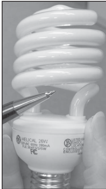
How much mercury exists in a CFL? It averages 5 milligrams or roughly equivalent to the tip of a ball point pen.
