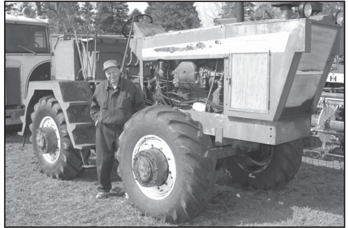
Floyd Knewtson, Madelia, started building his first tractor in 1970. It is 10 feet high, 16 feet long and 12 feet wide with duals. It has a two-cycle 426 cubic-inch diesel engine (equal to 852 cubic inches in a four-cycle).
