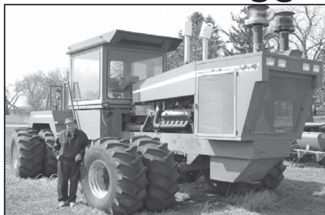
Knewton started building his second tractor in 1983. It is 13 feet high, 30 feet long and 14 feet wide with duals. It has a two-cycle 852 cubic-inch diesel engine (equal to 1,704 cubic inches in a four-cycle).
